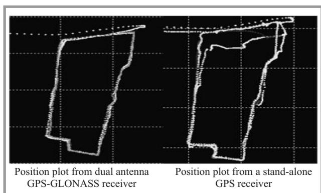
Fig. 9. Position trace from field test.
