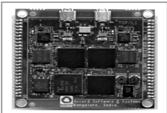
Fig. 7. Miniature dual antenna GPS-GLONASS receiver.
