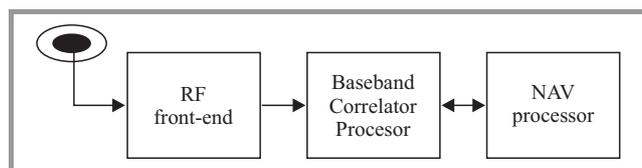
Fig. 1. Typical navigation receiver architecture.
