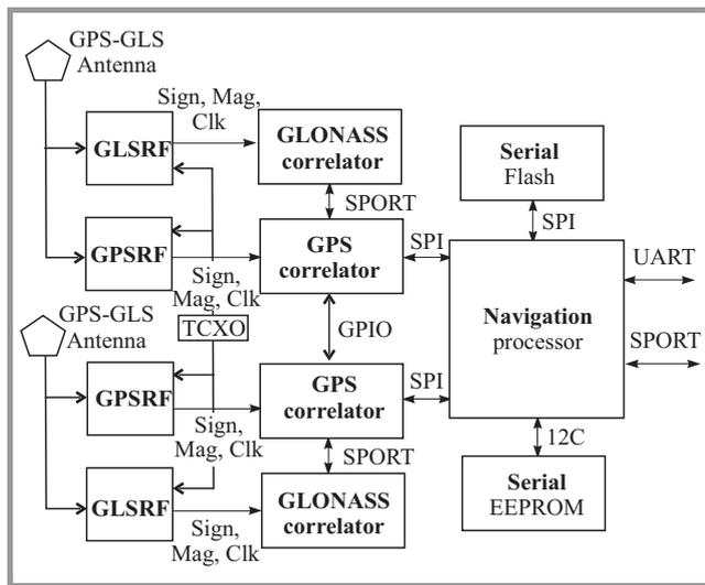
Fig. 2. Dual-antenna GPS-GLONASS receiver architecture.
