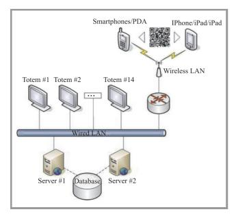
Fig. 3. QRouteMe installation setup.
