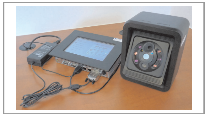
Fig. 10. Components of the developed station: a processing unit with a display for communication with a subject and an iris capture camera.
