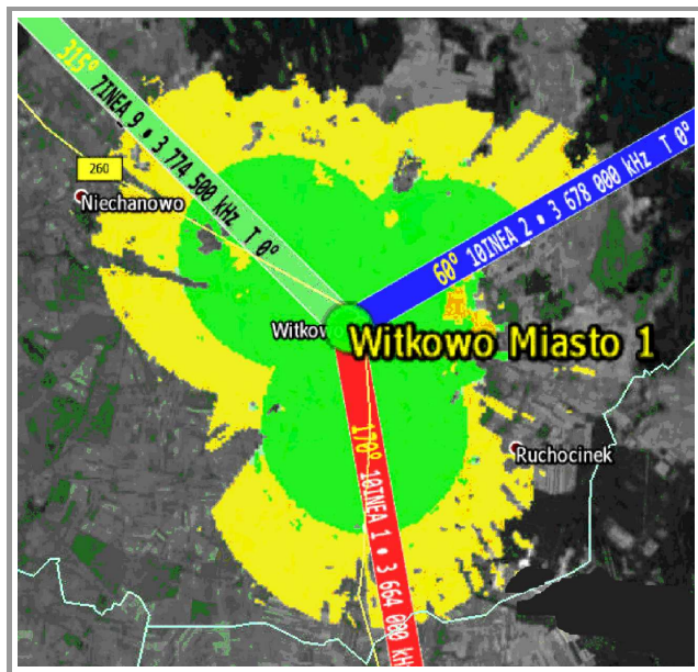
Fig. 4. Example of results of coverage prediction.
