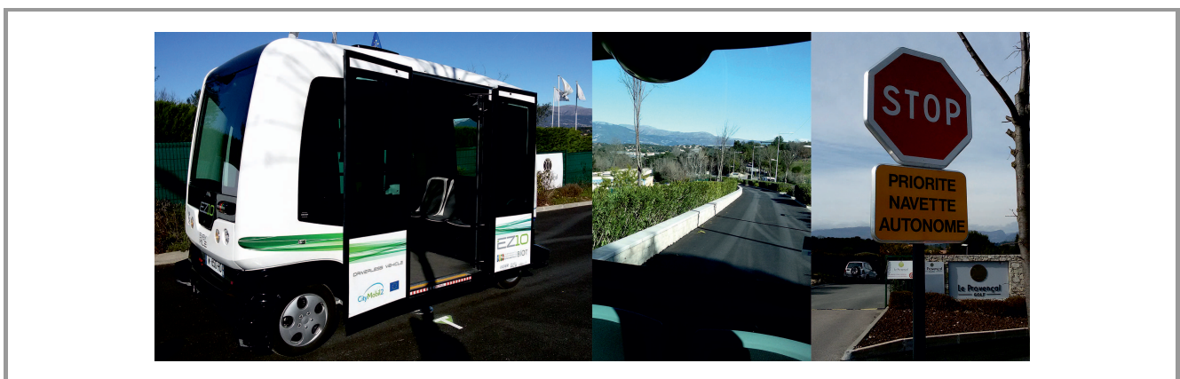
Fig. 5. EasyMile EZ10 (left), dedicated bus lane (middle), and autonomous vehicle precedence sign (right) (Sophia Antipolis, France, 2016).
