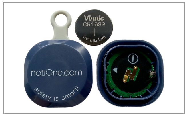
Fig. 4. Opened notiOne beacon with a CR1632 button cell battery.
