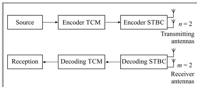
Fig. 9. Transmission system for STBC associated with TCM.
