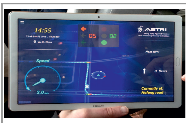
Fig. 4. LTE-V2X GLOSA demonstration by China Mobile, Huawei and ASTRI in the context of the 5G-DRIVE project.
