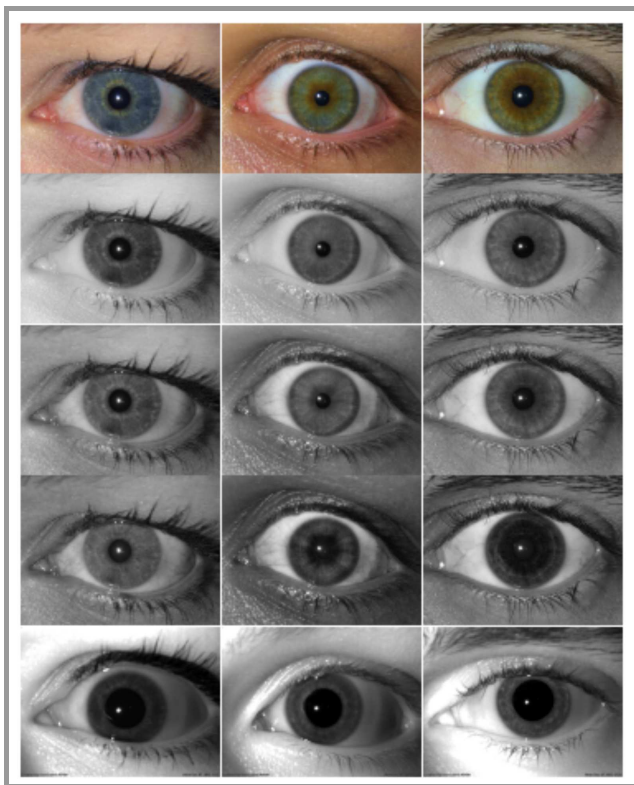
Fig. 1. Top row: cropped sample images obtained with the iPhone 5s: blue eye (left), green eye (middle), brown/hazel eye (right). Rows 2–4: grayscale versions of the images using red, green and blue channel of the RGB color space, respectively. Bottom row: NIR images obtained with the IrisGuard AD100. (See color pictures online at www.nit.eu/publications/journal-jtit )
