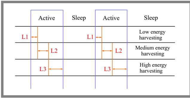
Fig. 3. Multi-layer structure for varying energy harvesting conditions.
