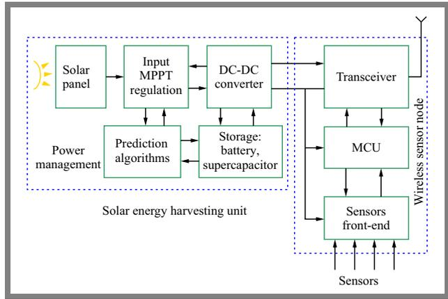
Fig. 5. Block diagram of solar energy harvester [26].
