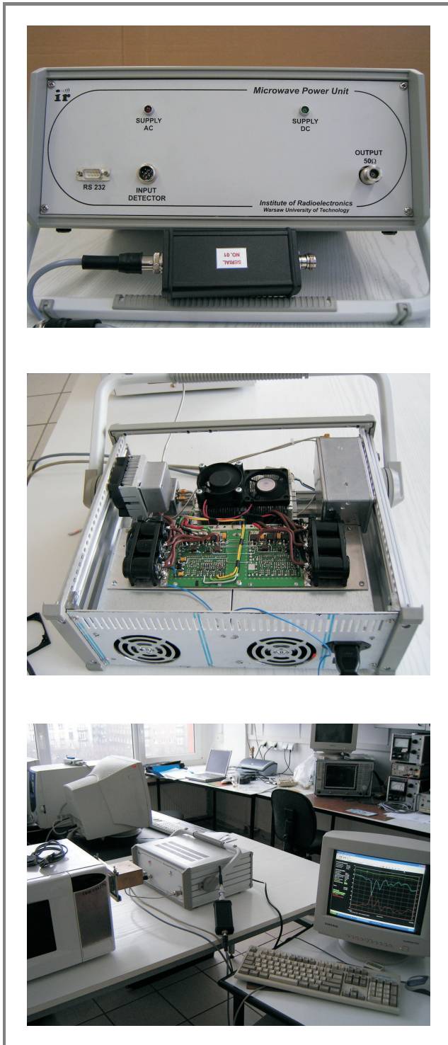
Fig. 9. The view of the 100 W ISM 2.4 GHz power test system.
