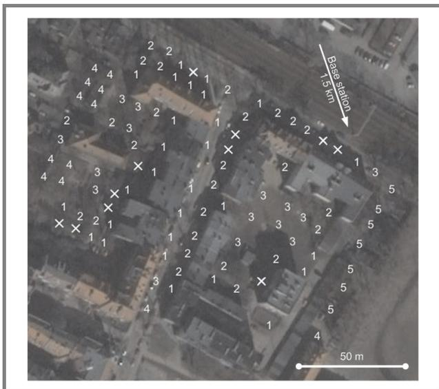
**Fig. 2.** WiMAX coverage hole effect: measured coverage of the WiMAX base station in 3.5 GHz band. Stable modulation profile chosen by client terminal: x – no communication; 1 – binary phase-shift key (BPSK); 2 – quaternary phase-shift key (QPSK); 3 – quadrature amplitude modulation 16 (QAM16); 4 – QAM64 1/2; 5 – QAM64 3/4.
