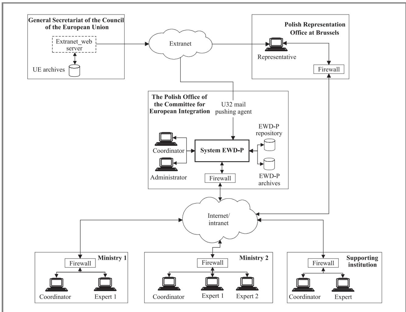
Fig. 1. The EWD-P system architecture.
