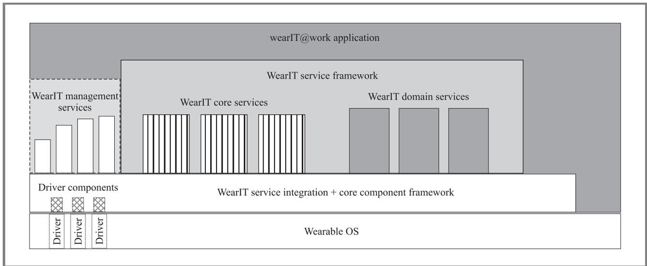
Fig. 7. General structure of the software framework.
