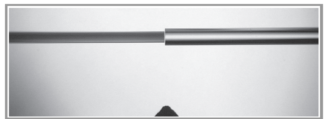
Fig. 2. Fibers cleaved and aligned with 10 \mu\text{m} gap (loss: 8.18 dB, electrode tip visible at the bottom).
