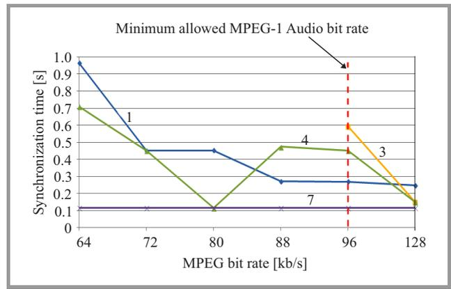
**Fig. 16.** Synchronization time as a function of MPEG-1 Audio bit rate for four phrases (1, 3, 4 – the same as in Fig. 1, 7 – speech) for a system embedding of a digital signature in an audio signal.
