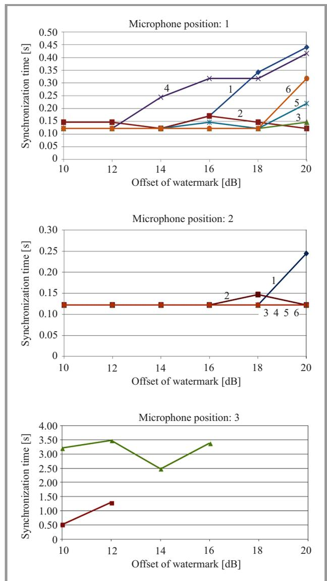
**Fig. 17.** Synchronization time as a function of watermark attenuation for six audio files same as in Fig. 1 for a system embedding of a digital signature in an audio signal.
