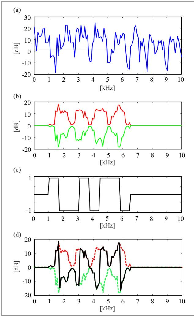
**Fig. 5.** The scheme of watermark embedding: (a) the cover signal  $\Delta \log |\bar{X}|$ , (b) maximal changes within the masking threshold  $\Delta^+ \log |\bar{X}|$  and  $\Delta^- \log |\bar{X}|$ , (c) the 6th Walsh function, (d) absolute value of the watermark in log-spectrum domain.
