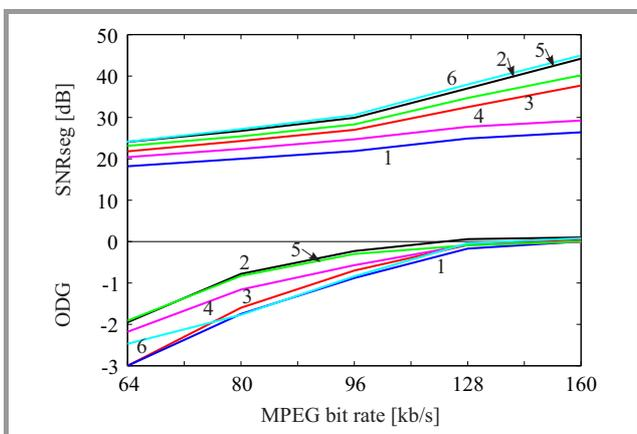
**Fig. 2.** SNRseg and ODG as functions of bit rate of the MPEG1-Audio codec for the same 6 audio files.
