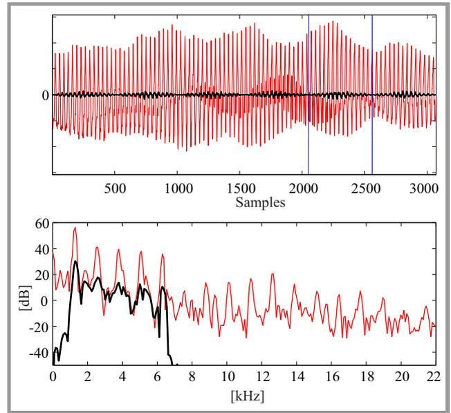
Fig. 4. The audio signal and the watermark (thick line) in time and frequency domain.
