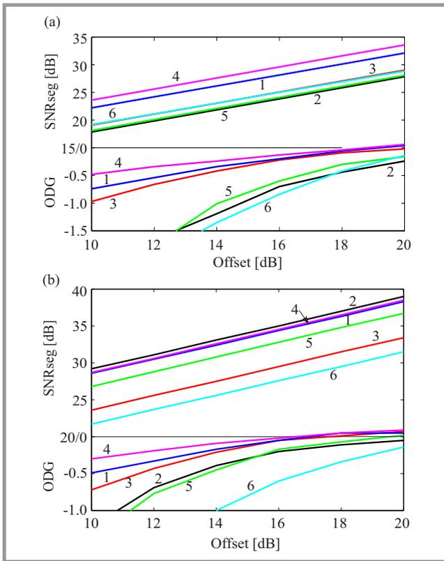
**Fig. 1.** Signal to watermark ratio (SNRseg) and ODG as functions of the watermark attenuation for 6 audio files: 1, 4 – songs; 2, 5 – piano with orchestra; 3 – violin; 6 – trumpet. Picture (a) concerns watermarking bit stream transmission, (b) with hiding of digital signature.
