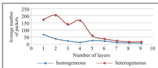
Fig. 5. Comparison of packets dropped for both networks.
