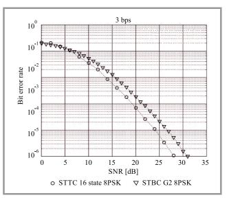
*Fig. 7.* BER versus SNR for spectral efficiency of 3 bps with only one receiving antenna.
