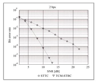
Fig. 11. Comparison between STTC and TCM-STBC proposed.
