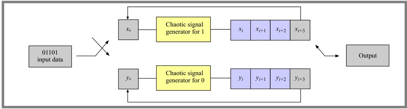
Fig. 3. CSK encoder proposed for error correction.
