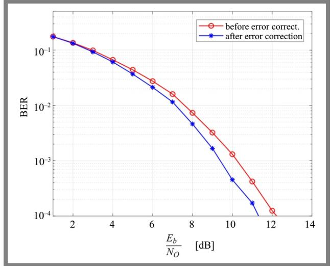
Fig. 11. BER after and before error correction,  $N_d = 4$ .
