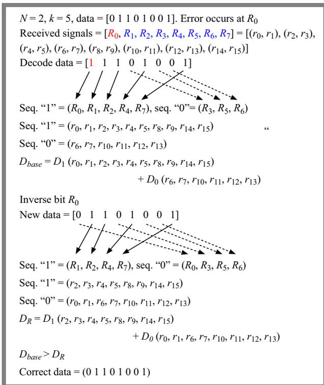
Fig. 8. Error correction algorithm method from [14].
