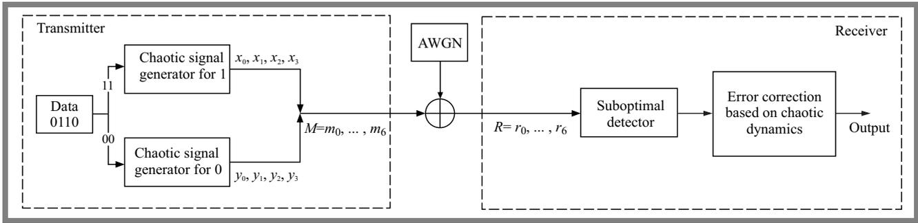
Fig. 1. CSK system with the proposed error correction coding scheme.
