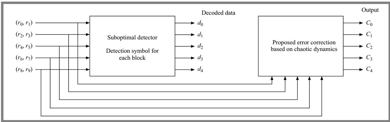
Fig. 6. Error correction algorithm diagram.
