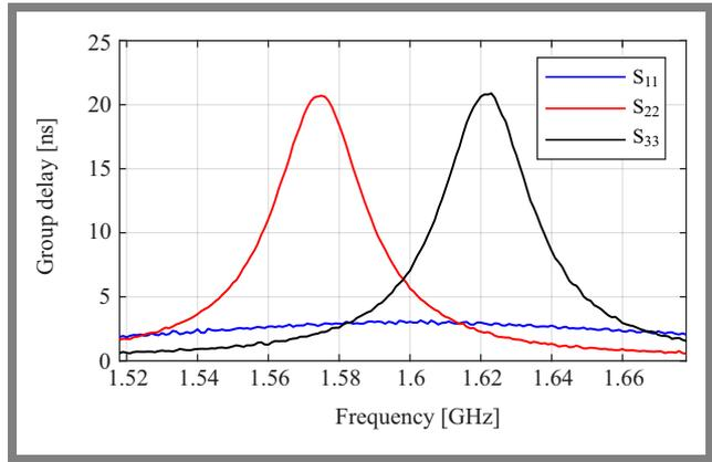
Fig. 4. Group delay measured at the three ports.
