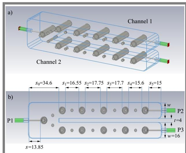
**Fig. 1.** Model of the diplexer: a) perspective and b) top views. The dimensions (in mm) are: the coaxial inner (outer) diameter is 5.5 and 7.3, the screw diameter is 3, the coaxial cable inner and outer diameters are 1.27 and 4.1, respectively. The heights of the tap points from the bottom of the cavity are 18.75 for P1, 6.75 for P2, and 6.90 for P3, respectively. The radius of the fillets is 4.
