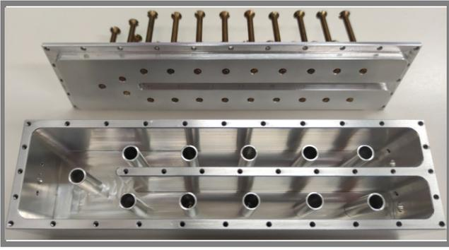
Fig. 3. Manufactured diplexer.
