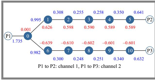
**Fig. 2.** Topology of the diplexer. The blue circles indicate the resonators, while white circles stand for ports. The numbers in red indicate normalized resonant frequencies  $m_{i,i}$ , while those in blue indicate normalized coupling coefficients  $m_{i,j}$ . The white numbers indicate the number of resonators.
