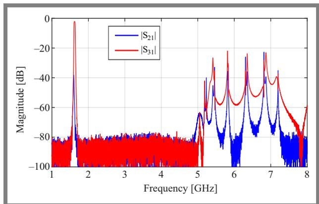
Fig. 6. Measured wideband response in the range 1–8 GHz.
